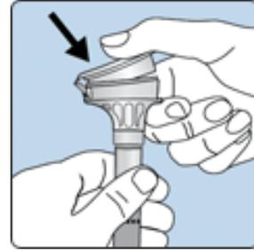
5. Continue holding the tube upright, and unscrew the funnel lid from the tube.
